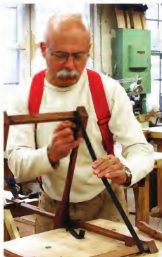
Clamp in position. Leg assemblies are clamped to the bench before webbing is tacked to the upper rails to hold the legs in the open position.
